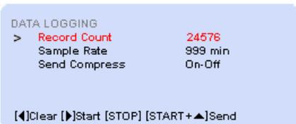
[◀]Clear causes the Record Count to become zero, [▶] Start causes logging to begin, [STOP] halts periodic sample acquisition, and [START+▲] causes all log records to be sent from the RS232 serial port.
